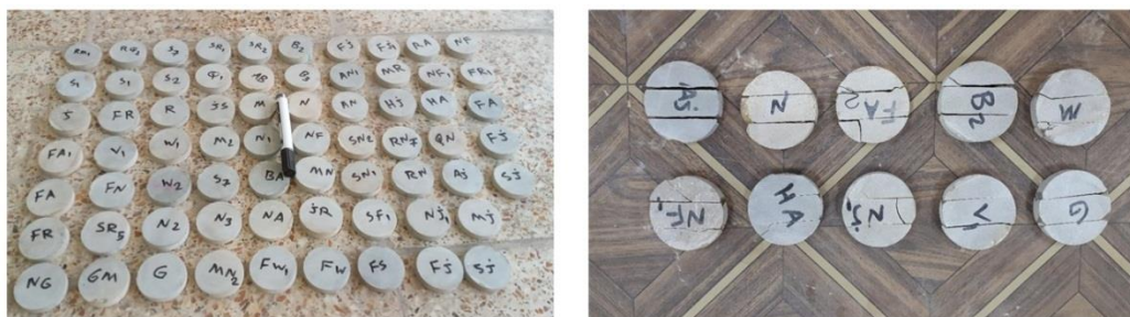
Figure 4. Some of specimens before and after failure in the BPI test
