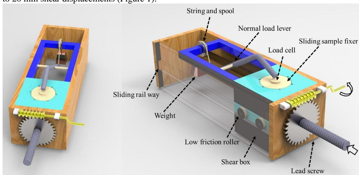
**Fig. 1.** conceptual model of a portable tribometer for measuring residual friction coefficient of rocks.
