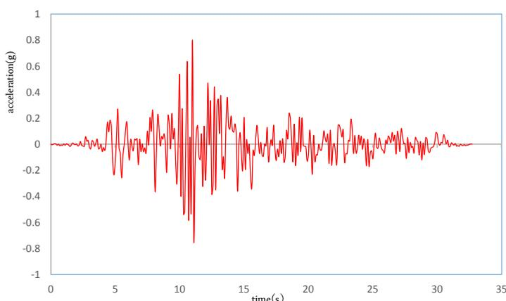
**Fig1.** Accelerogram used in Dynamic Analysis of Azadi Dam (Tabas Earthquake)
