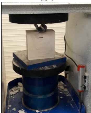
Fig 5. The uniaxial compression test with sample set up.
