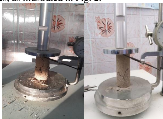
Fig 2. Uniaxial compression tests on the treated samples
