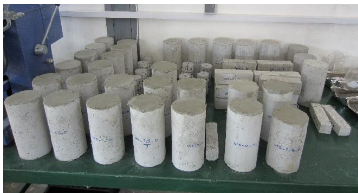
Fig. 1. Prepared specimens for uniaxial compression, Brazilian tensile, and three-point flexural tests
