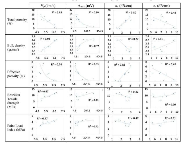
Table 1. Correlations between physical and mechanical properties and ultrasonic parameters
